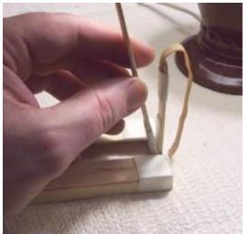
Test the movement of the catapult arm by moving it up and down. It should move freely. This is why we leave the little space between the black lines. It acts as a hinge.
