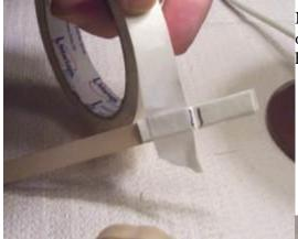
Now pinch the free ends of the tape together so they stick to each other. And wrap at least three wraps around the stick so it all holds together nice and tight.
